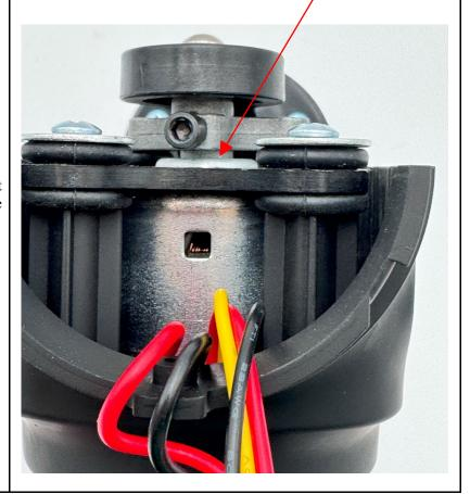
The drive mechanism of the accused product comprises a flywheel operatively connected to the output shaft of the motor to rotate about a flywheel axis, the output shaft extending into the flywheel along the flywheel axis:
