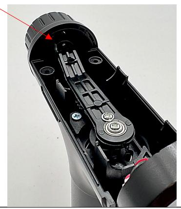
In the accused product, the motor is configured to cause the piston to reciprocate at a first speed.
