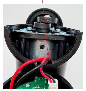
a motor operatively connected to the proximal end of the piston,
